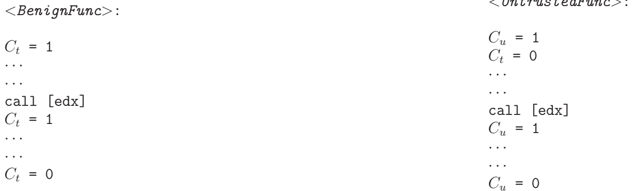
Figure 2.2: Scheme showing the points at which context flag bits are set and reset in a trusted function BenignFunc and an untrusted function UntrustedFunc . If only C_t is set, the program is in trusted context. If only C_u is set, the program is in untrusted context. If both bits are set, the program runs in trusted context on behalf of the untrusted code.
